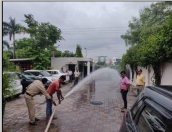
Fire Safety: Fire Hose Reel Pressure Test
