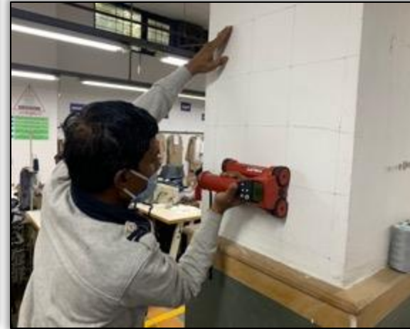
Structural Safety: Ferro-Scanning Test
