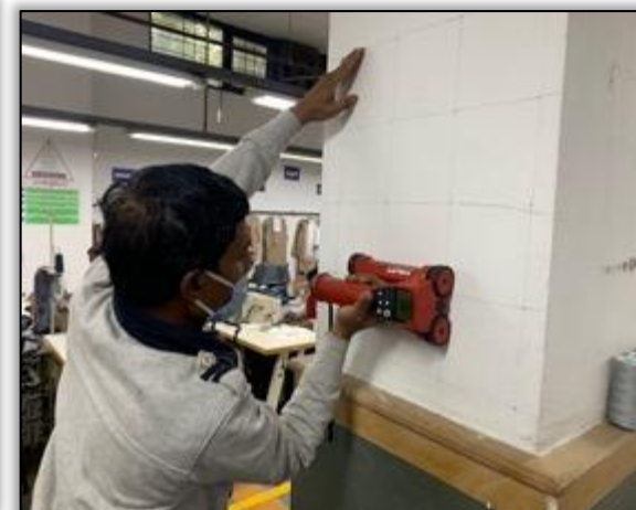
Structural Safety: Ferro-Scanning Test
